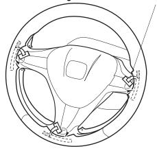
Thread the lacing string into the needle. Make inclined stitches in the back of the steering wheel cover up to the hole that is right above the spoke as shown.
