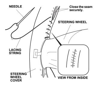
8. Keep lacing while adjusting the steering wheel cover so the seams on both sides of the steering wheel are aligned.
